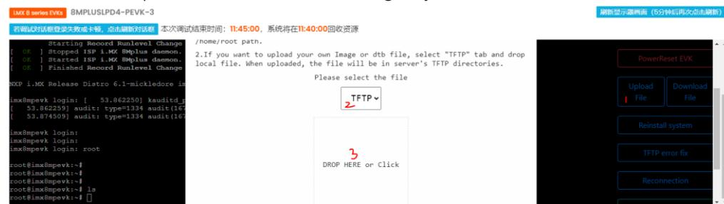
Then click the PowerReset EVK button to restart the development board. You can see the following printout. This can be used as a debugging method.
